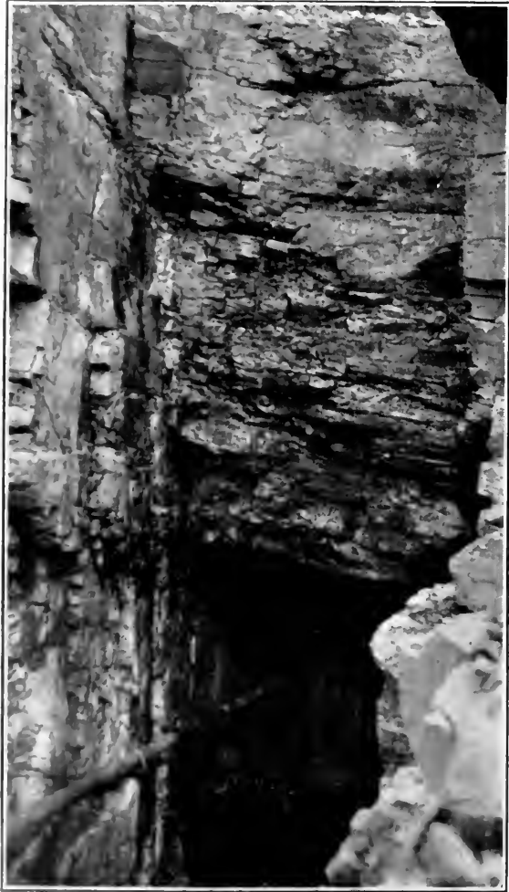
A cut on silver-smaltite vein in Huronian sediments. La Rose Mine, Cobalt.
